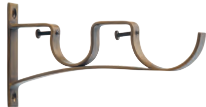
Harlan Double Bracket QS214HADBK 3 3/4" H x 3/4" W backplate, 6" front return and 2 1/2" back return, front cradle holds 2 1/4" DIA pole, back cradle holds 1 3/8" DIA pole Metal, Antique Brass
