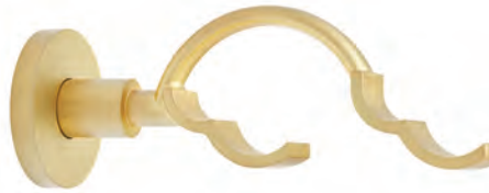
new Talon Double QS138TADBK 2 1/2" DIA backplate, 6 1/2" front return and 3 1/2" back return, 3/8" clearance above backplate, use with Calla C-Rings Metal, Satin Gold
