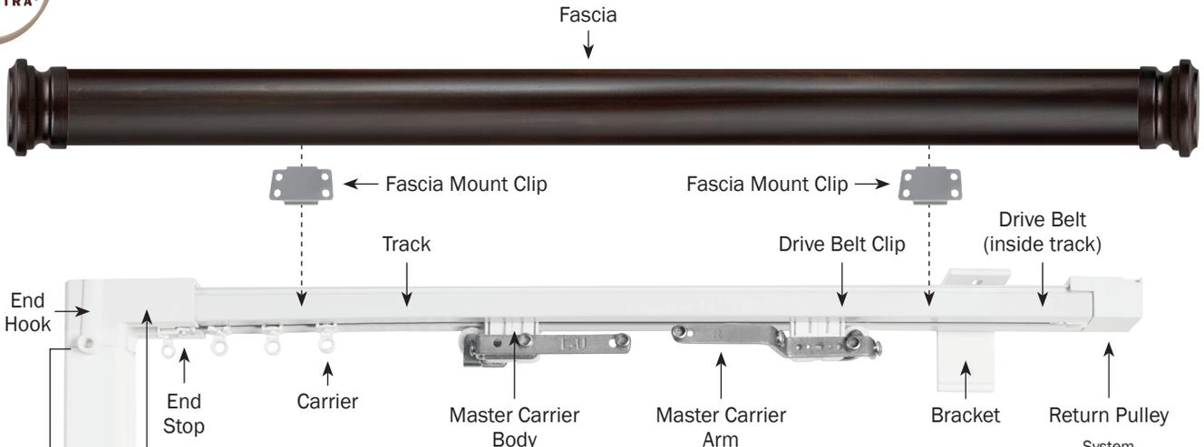
System Requirements: 1 Drive Pulley & 1 Return Pulley for One-Way Draw; 2 Drive Pulleys for Center Draw.
