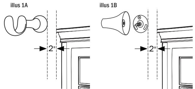
3. If using plastic expansion anchors, pre-drill holes using 3/16" drill bit. If drilling directly into a stud or wood trim, pre-drill holes with 3/32" drill bit. Attach the bracket mounting base using the screws provided.
