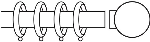
8. Attach the finials to the pole and tighten the set screws with the Allen Wrench provided on the finial base by hand to complete the finial installation. **NOTE:** Some finials may have an inset screw in order to tighten it to the pole. For those designs, use the Allen Wrench provided with those finials.
